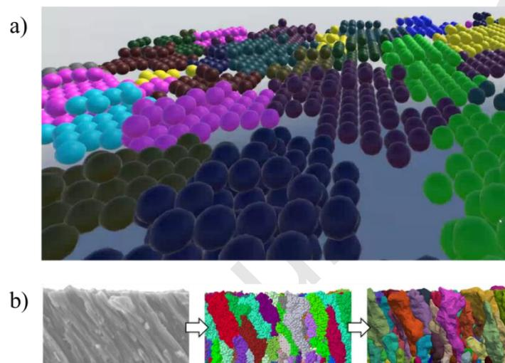
**Fig. 10.** Film growth: a) atomic view; b) columnar view [20].
