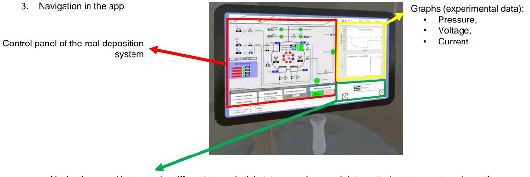
Navigation panel between the different steps: initial state, pumping, gas inlet, sputtering, transport, and growth. + return to the main Menu
